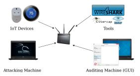
Fig. 2. IoT testbed components
